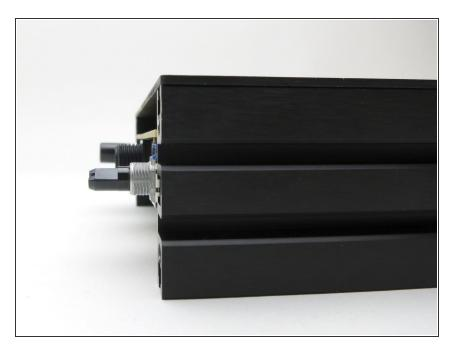
The PCB, top plate, and PCB will all be flush with each other.
