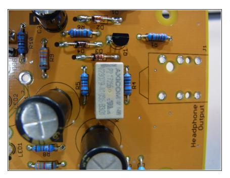
The relay fits on the board as shown. It's pins are keyed and cannot be installed backwards
