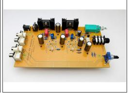
Make sure all these components are sitting on the PCB low and square, failure to do so will result
