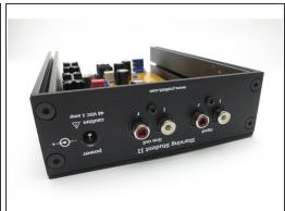
Rear panel attaches with black countersunk screws.
