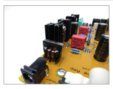
The common mode choke can go into the PCB either way – orientation doesn't matter. Put it in the PCB and solder. You don't need to trim the leads.
