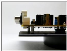
The PCB will be slightly behind the side rails, and the top plate will hang over both the PCB and rails.
