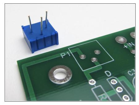
The potentiometers have three leads in a triangular formation, they are impossible to insert backwards.
