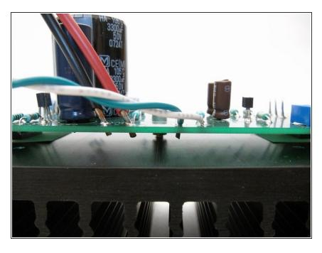
Since many wire connections need to be soldered from the top of the PCB, strip the insulation and trim so it sticks through only 1-2mm. Make sure it does not touch the heatsink!
