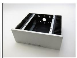
Sheet metal screws attach the top and bottom panels
