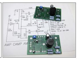
Complete stuffed PCB shown here. Note transistor and capacitor alignment.
