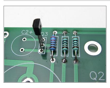
Place Q3. ZTX450 Like the other small transistor the flat of the transistor package matches the flat of the silkscreen.
