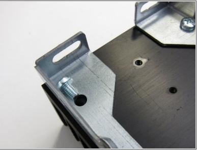
Attach the rails to the heatsinks
