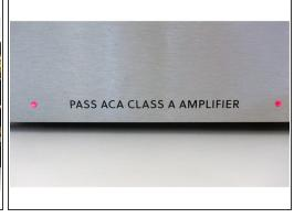
The LEDs are routed forward and placed in the front panel hole - the wire stiffness will keep them
