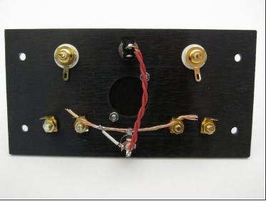
Power to the switch. Again, be careful to trim and clean up any wire after it's soldered.
