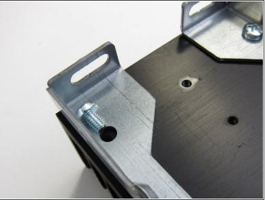
Attach the rails to the heatsinks
