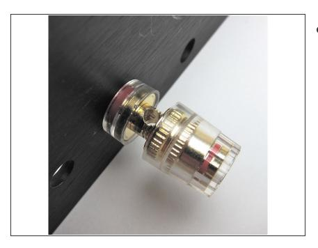
Align the hole in the post to be vertical.
