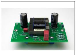
Front end board for P-Channel amp.
