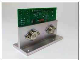
The P channel output board comes partly assembled and tested by Nelson Pass himself.
