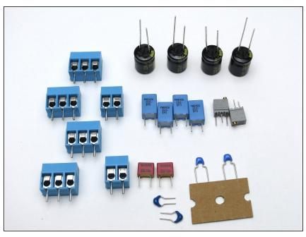
Please note the 10pF capacitors are the two on the tape, the 5pF are loose.
