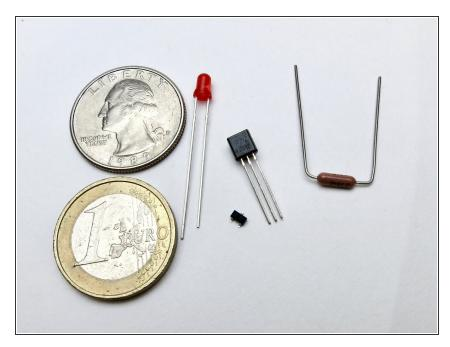
Yes, the SMD transistors are very small. It's not a big deal though, we'll show you how to position and secure them for soldering in the next step.
